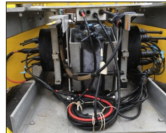
Telemetry and control bottle
