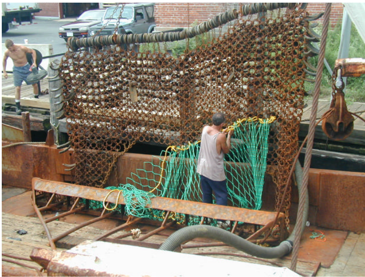
Figure 7. Crewman sewing a twine top into a scallop dredge. This procedure takes about 30 – 45 minutes at the dock or in good weather.
