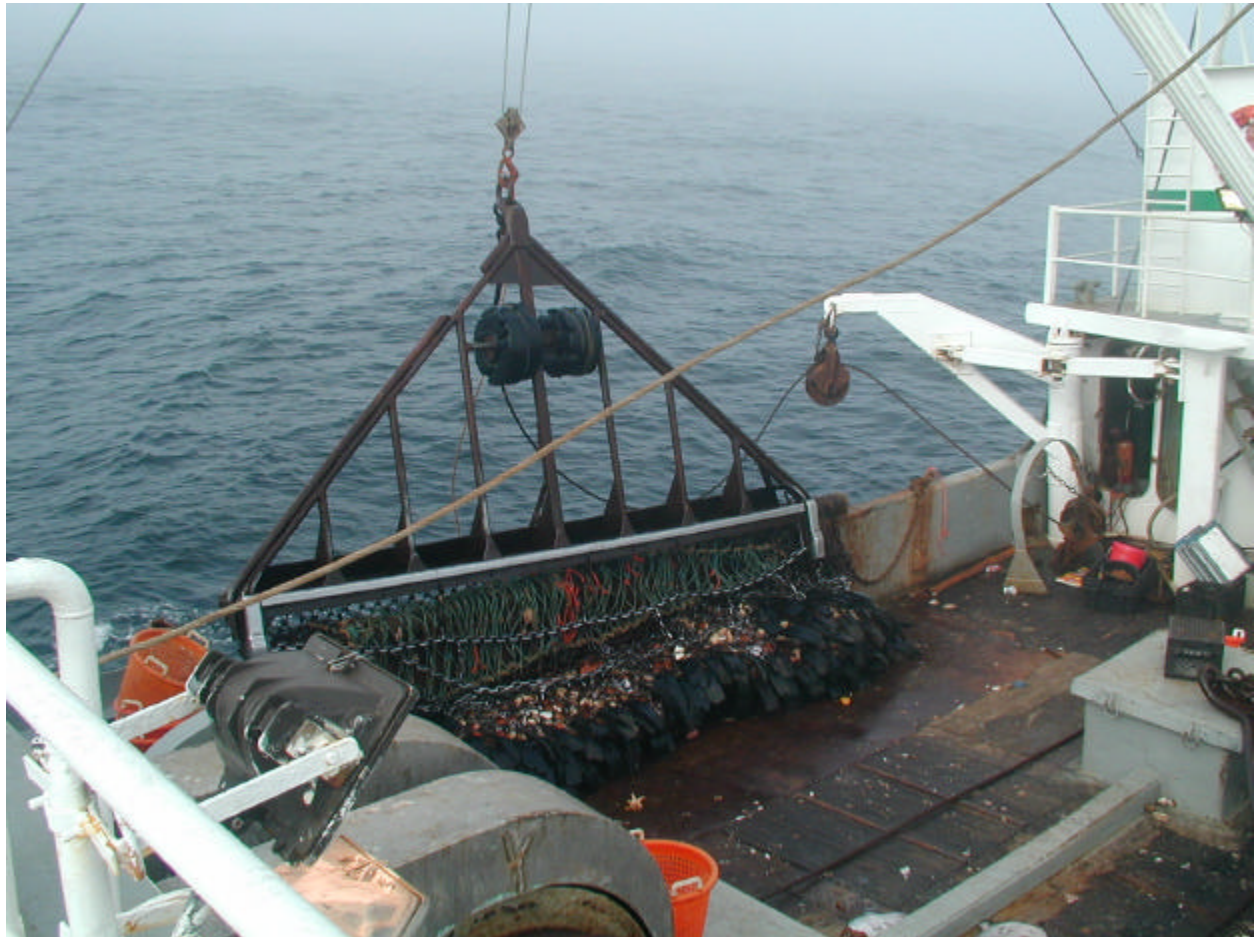
Figure 8. Bail of a scallop dredge. The frame acts to keep the dredge bag spread wide and on the bottom. Note the shiny part of the bail that keeps contact with the bottom, versus other portions of the bail that do not.
