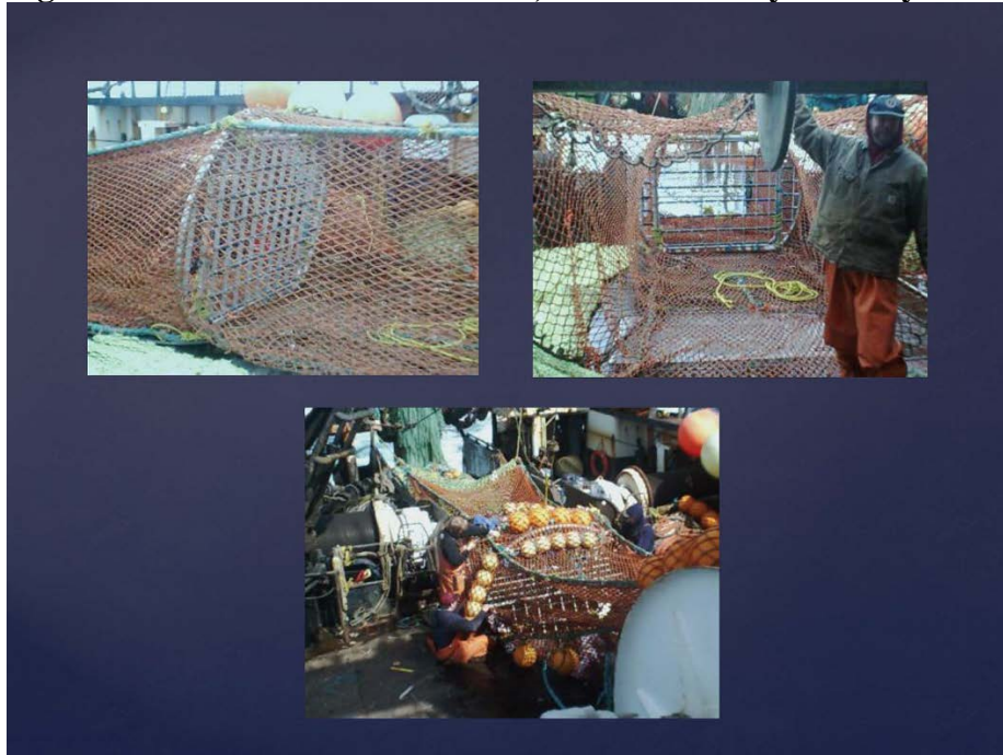
Figure 6 – Halibut Excluder Device with Kites, Presentation by Bill Hayes at Trawl Gear Workshop
