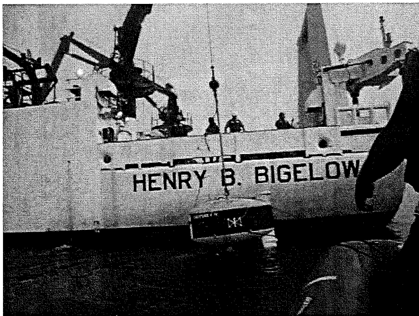
Figure 6 Odyssey IV AUV during hoist being assisted by personnel aboard Henry B. Bigelow's rescue launch.
