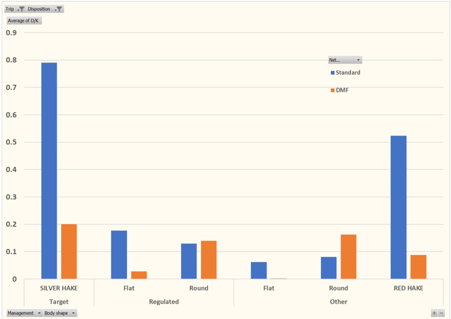
Figure 17. Comparable catches of silver hake (target), red hake, regulated multispecies, and other species by body shape for six raised footrope trawl/control trials in 1994. Data from Carr 1996, used with permission of MA DMF.
