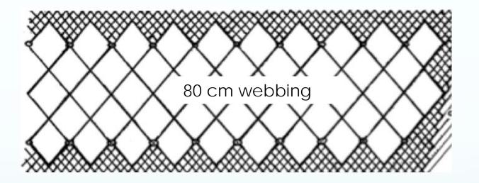
The large mesh panel is made of 80cm (32") mesh 6mm poly webbing, 2 meshes deep X 16 meshes wide sewn into the standard 16cm (6") mesh of the belly. With the 'saw-toothing' of the 16cm mesh, this yields an effective opening of 3 full meshes deep, a total of about 8' of large mesh. The panel attaches five 16cm meshes (approx. 2.5') behind the footrope and goes from gore to gore (22 meshes wide or approx. 30').
