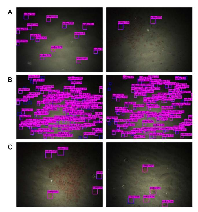
Figure 21. Sample output images from the Scallopscan YOLOv3 test set. Overlaid blue boxes are manual annotations and pink boxes are neural network detections. Each detection is labeled with a confidence value. Examples are shown of images where (A) counts between annotators and Scallopscan agreed, (B) Scallopscan missed scallops that were crowded, obscured by sediment, or located on the perimeter of the image, and (C) Scallopscan detected scallops that were inadvertently missed by annotators.
