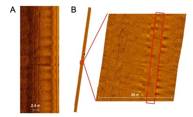
• <u>Figure 6.</u> (A) Example of a scar left behind by the 2.4 m (8 ft) survey dredge visible in a single raw side-scan sonar file. (B) The complete side-scan sonar mosaic from a mission with a section selected and enlarged to depict the dredge scar, highlighted with the red box.
