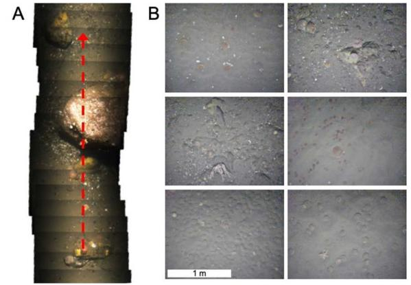
• Figure 5. (A) A sample "filmstrip" of raw images with the direction of AUV travel indicated with the red arrow. (B) Sample enhanced images collected in the Nantucket Lightship Closed Area during this study, displaying the range of scallop densities and substrate compositions encountered.
