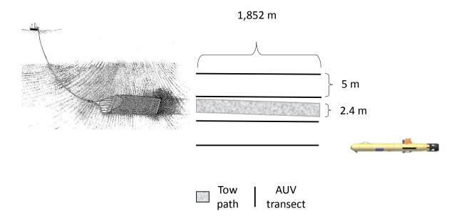
• <u>Figure 3.</u> Schematic of a paired survey dredge tow/AUV mission for a selected site, with a dredge tow, number and length of AUV transects and spacing between AUV transects. 2.4 m is the width of the survey dredge frame. Credit for image of vessel and dredge https://njscuba.net/artifacts/obj\_dredge-trap.php
