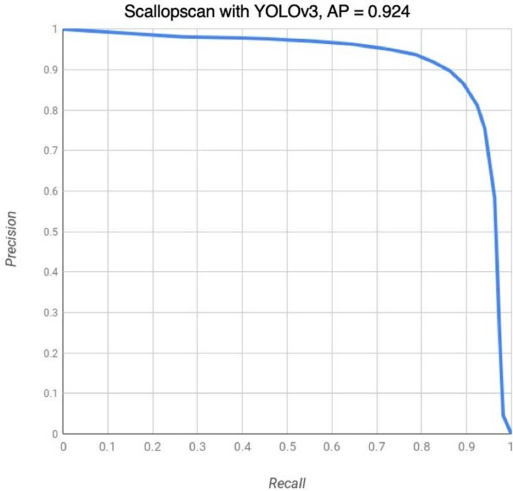
**Figure 20.** The precision-recall (PR) curve for Scallopscan with the YOLOv3 architecture trained for 20,000 epochs. The curve was generated from a test set consisting of 72,879 scallops from 19,469 images. Average precision (AP) was 0.924 for this image set.
