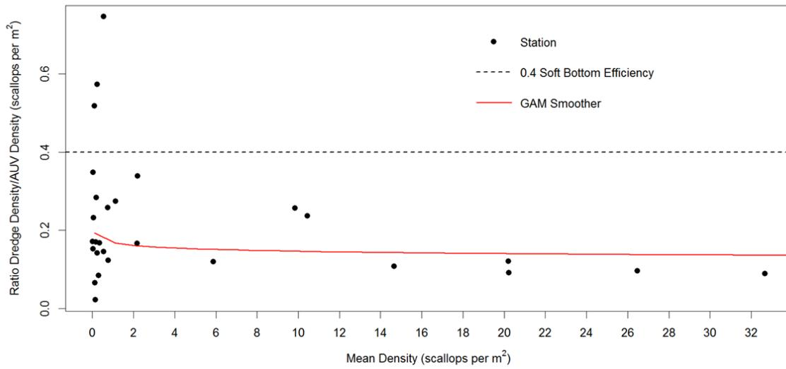
**Figure 29.** The ratio of dredge density to AUV density (scallops per m<sup>2</sup>) plotted against mean density (dredge and AUV) by station. The black dashed horizontal line is the assumed soft bottom dredge efficiency of 0.4. The red curve is the GAM smoother.
